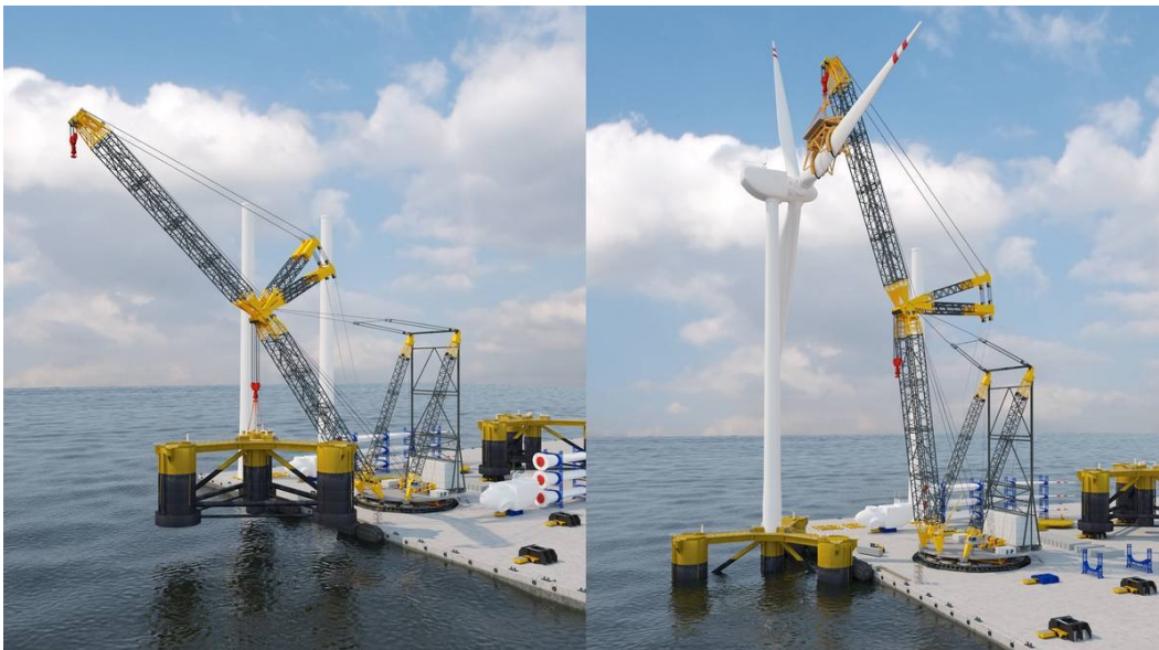
FIGURE 10: RING CRANE, SOURCE: MARINE LINK
