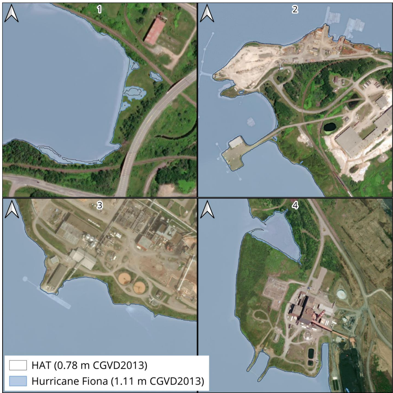
Figure 4-4: Flood extents in the project area for Hurricane Fiona static flood elevations. Tidal elevation as occurred during storm event. Figure shows flooding details in key areas.
