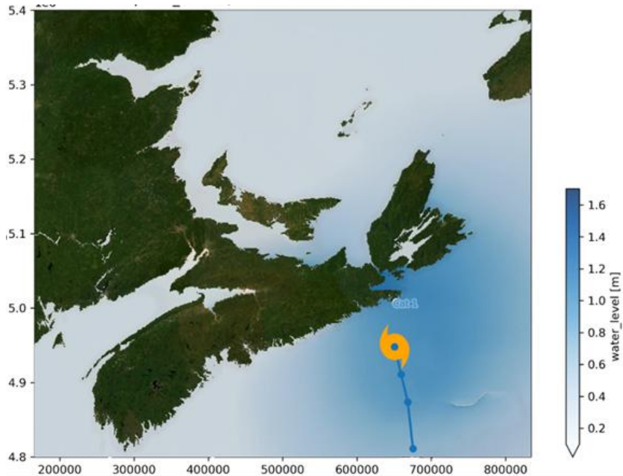
Figure 3-11: Residual storm surge generated by Hurricane Fiona using the SFINCS numerical model. Water level changes in this figure are due to modelled storm surge.
