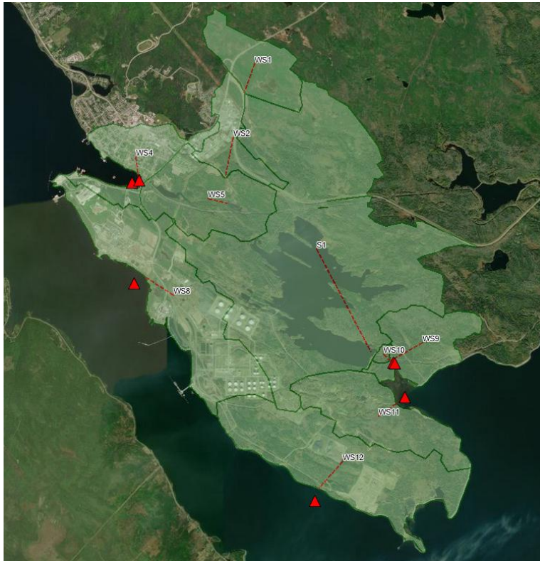
Figure B-1: Hydrological model layout for study area watersheds. Red triangles indicate locations where flow time series are generated to serve as inputs for the coastal model.
